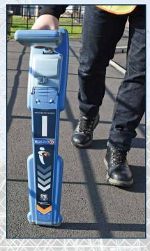
Shifts the locate frequency to survey in areas prone to interference or where more than one operator is working.
