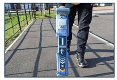
Swing Warning System Alerts the operator of excessive side to side movements, driving correct RD8200 usage.
