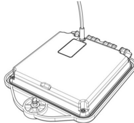
Figure 4.13 Charging the transmitter Li-Ion battery pack
