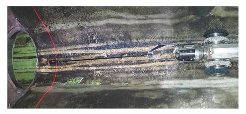
The advanced variable laser profiler allows the operator to control the size of the laser ring, making it suitable for a wide range of pipes. The profiler diode provides a laser ring that is suitable for pipes beginning at 4" / 100mm and powerful enough for pipes greater than 1 metre (3 feet) in diameter.
