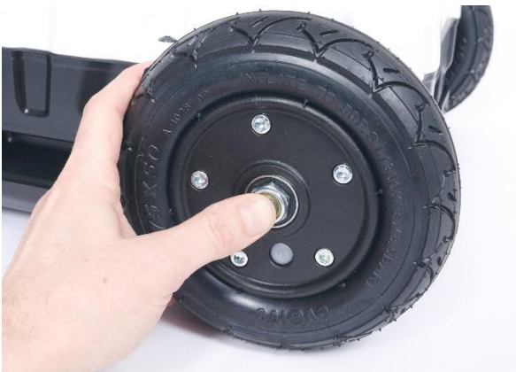
Press the quick-release pin and pull the wheel to remove it.
